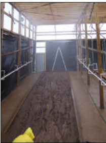
ASTM D 6459 Slope Testing Facility (bare soil test shown)
