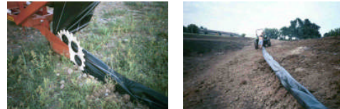
Slicing is Quicker, Cheaper, and Less Prone to Undermining
