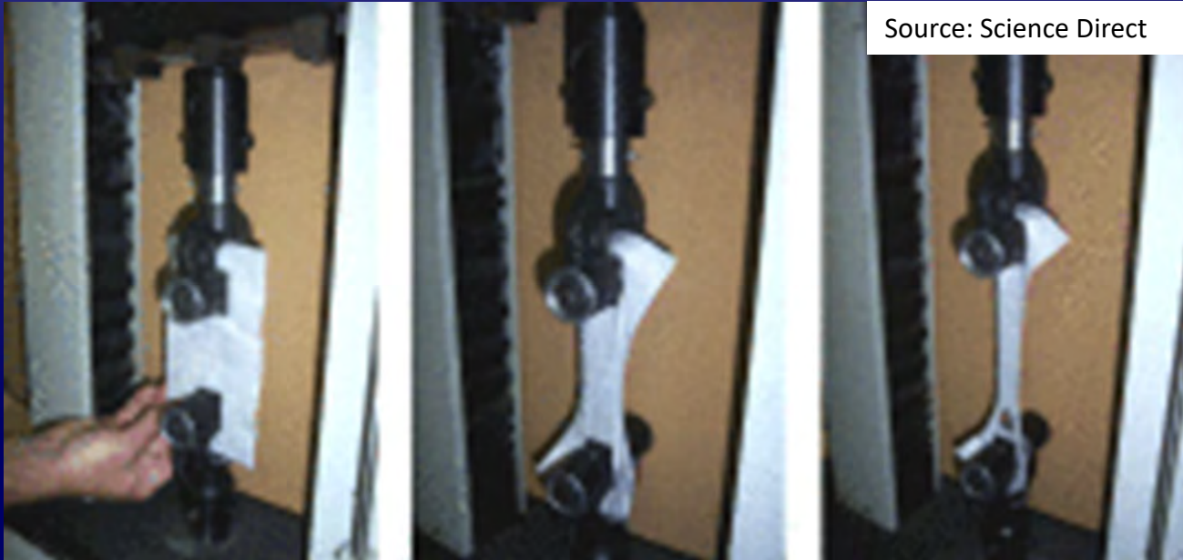
Note edge effect – elevated tensile strength
