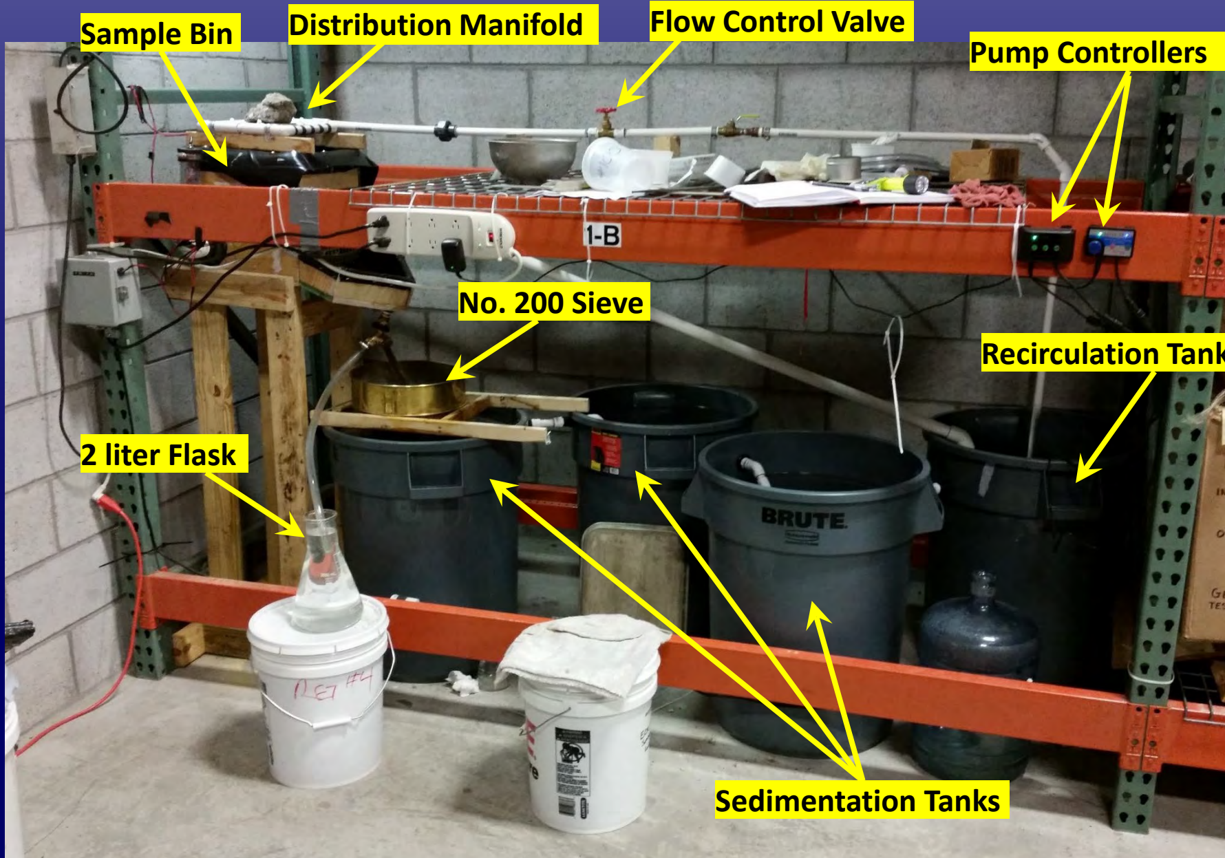
Test Apparatus – Geotextile for Pavement Base Drain
