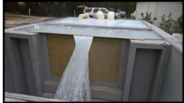
Figure 2. V-notch Weir in Headbox
