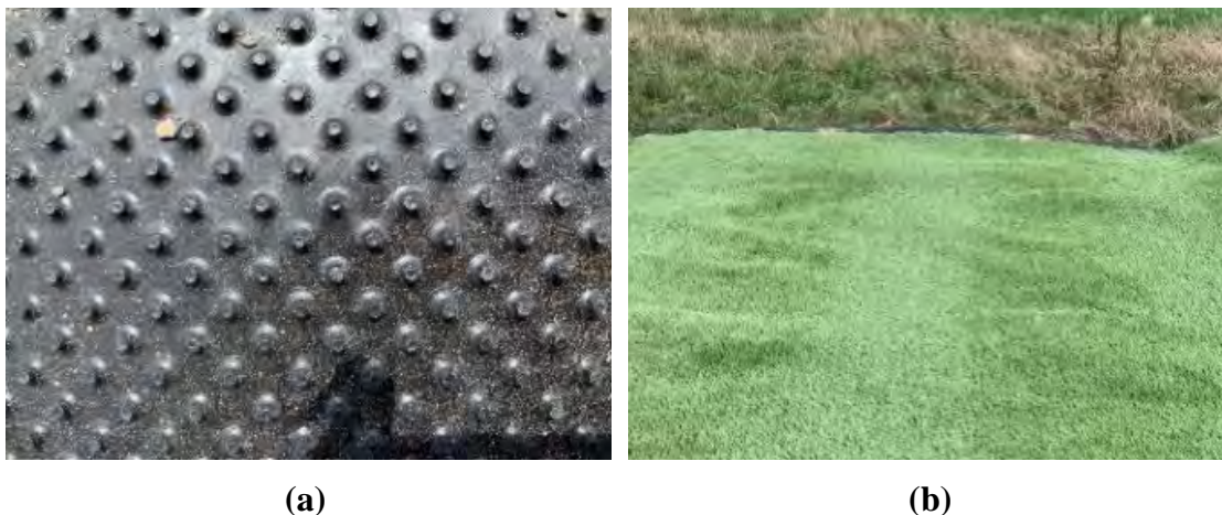
Figure 2. (a) Textured geomembrane layer (b) engineered turf.
