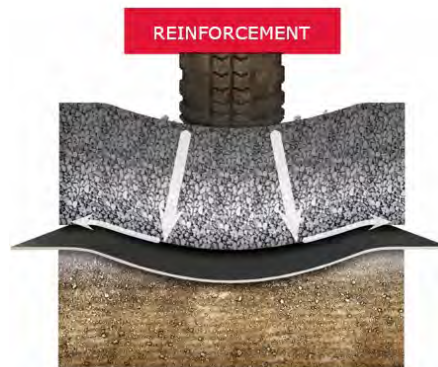
Figure 2. Mechanism of reinforcement – membrane effect.
