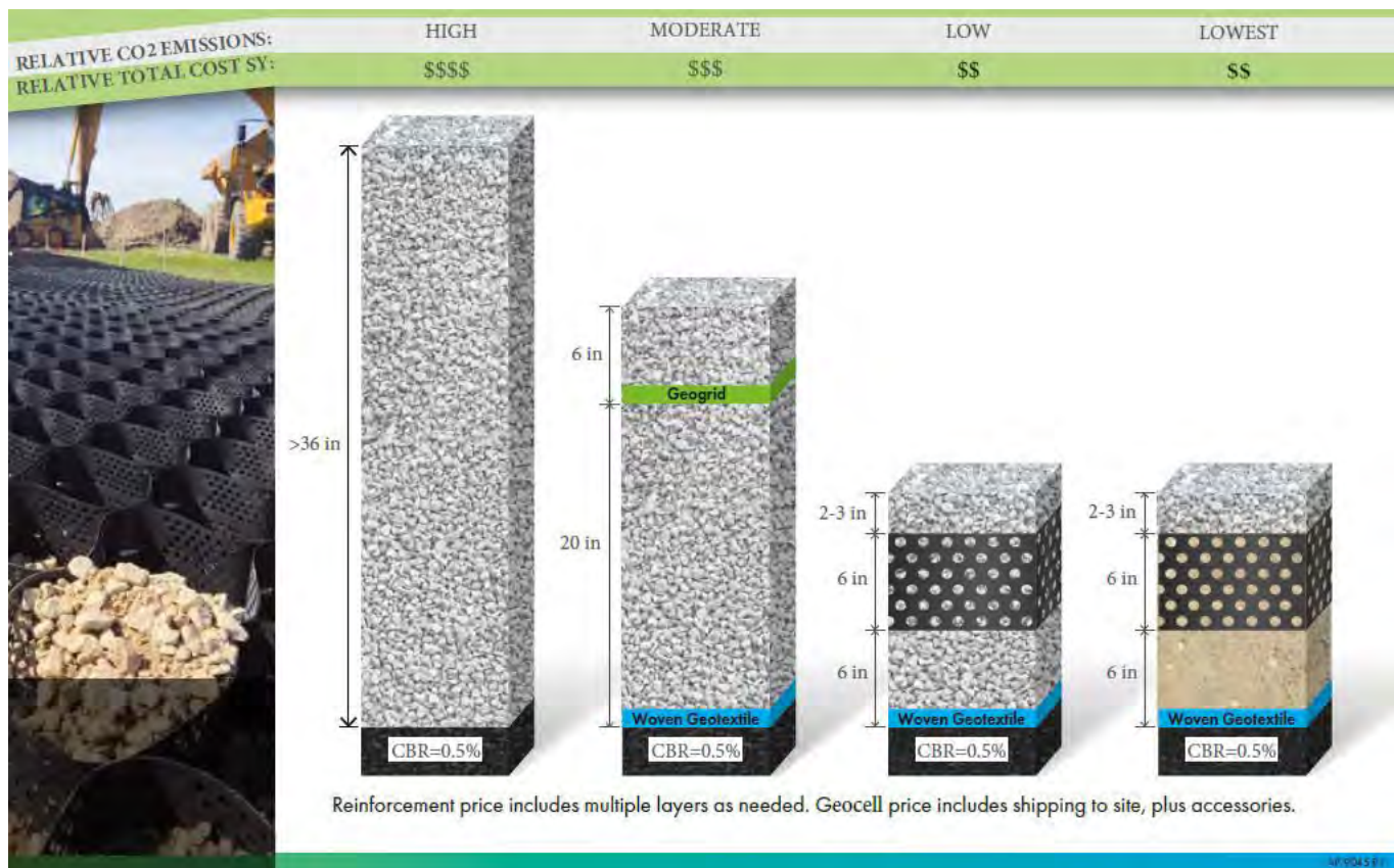
Figure 6. Load support cost-benefit comparison (Presto Geosystems 2022)
