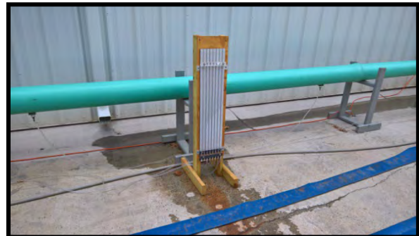
Figure 4. Monometer Board for Reading Piezometric Heads
