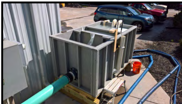
Figure 7. Headbox and Weir with attached Stillwell for HOBO logger
