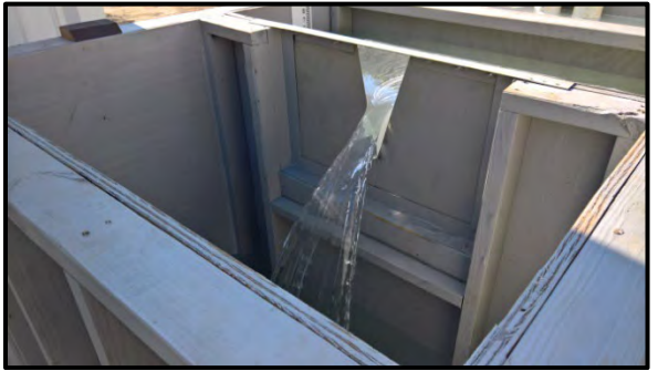
Figure 6. 33° V-Notch Weir used for Lower Flow Testing
