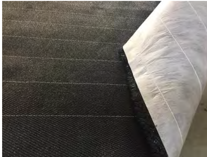
Figure 9. Geotextile tube with nonwoven filter inner liner.
