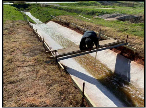
Figure 16. Depth Measurements used a Point Gauge
