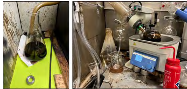
Figure 10. Bitumen extraction test.
