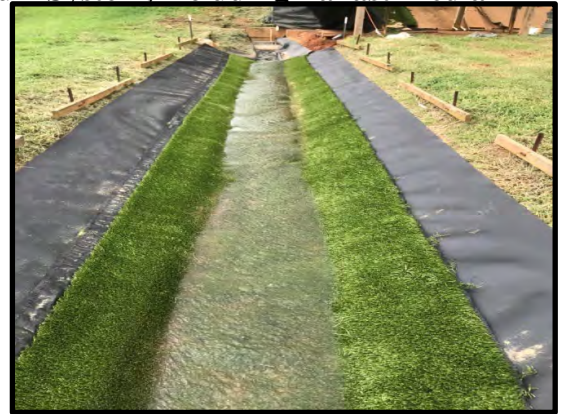
Figure 19. Uniform Flow in Turf-lined Channel
