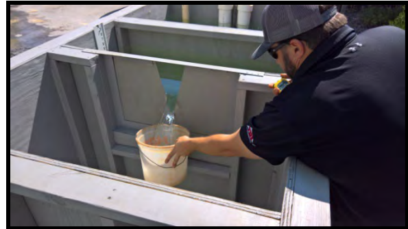
Figure 8. Example of Timed Catch to Verify Flow Rate
