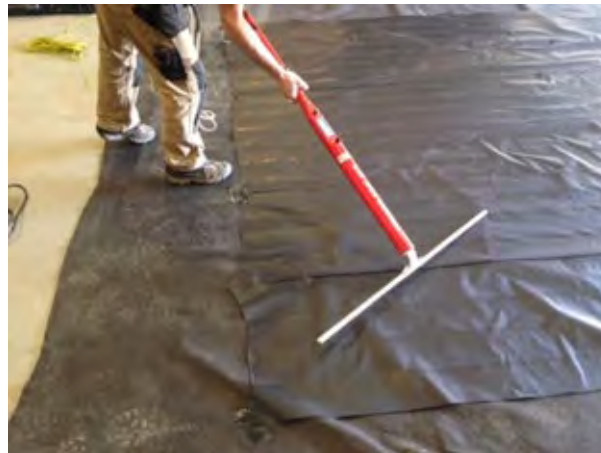
Figure 2. Arc testing on a 3-mil conductive film.
