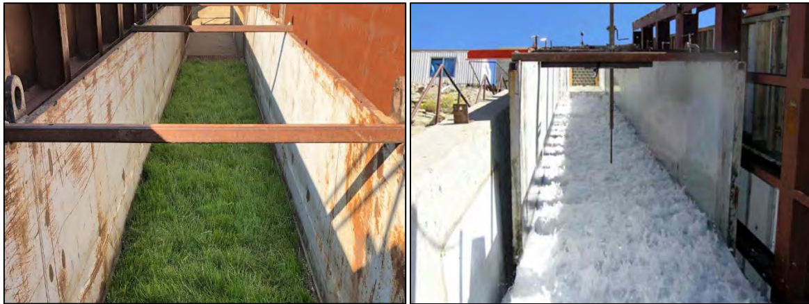
Figure 3. Full Scale Testing per ASTM D-6460 – Vegetated HPTRM (Left) and during Flume Test (Right)
