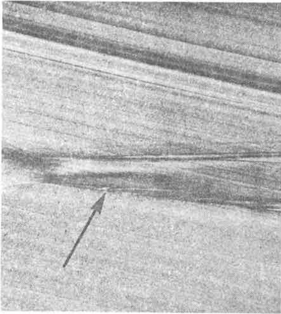
FIGURE 8. Residual stress (arrowed) in hot wedge seam. (x 65)
