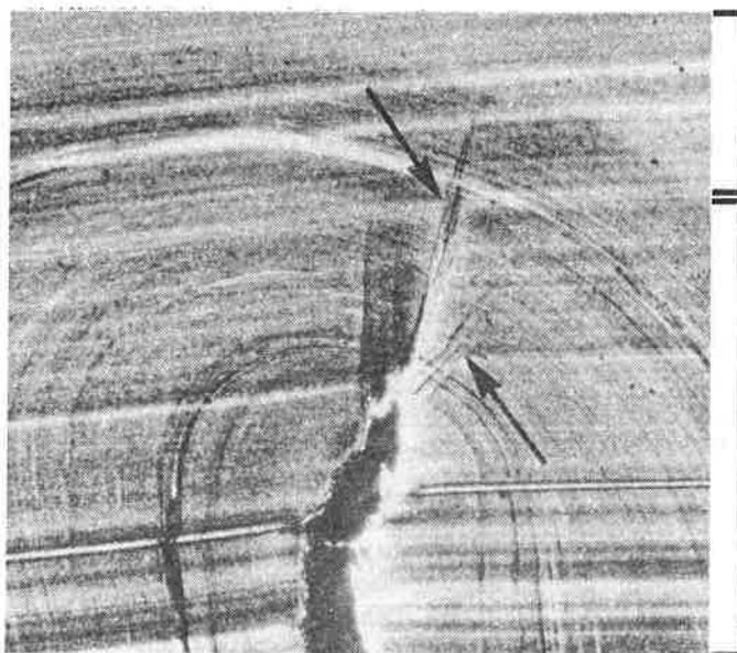
FIGURE 12. Arrow indicates cracks and crazes extending up from a crease in the bottom geomembrane. (x 65)
