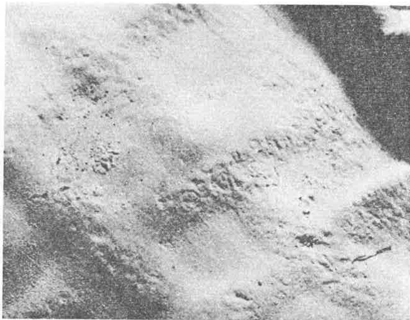
Figure 7. Close-up of scrim pattern; 1.1-mm CSPE (11.5X).
