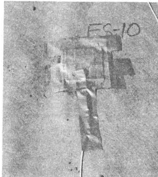
Photo 2: Installation of Strain Gauge for Typar 3601 Fabric
