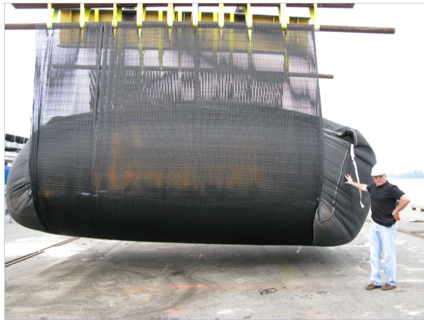
Figure 2. 90 Ton Geobag Lifted With 400 kN/m Geogrid
