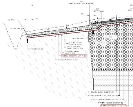
Figure 2. Cross section of the apron
