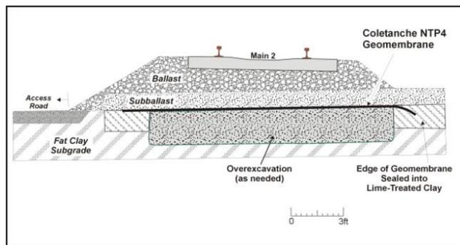
**Figure 5. Design Cross Section for BNSF**
