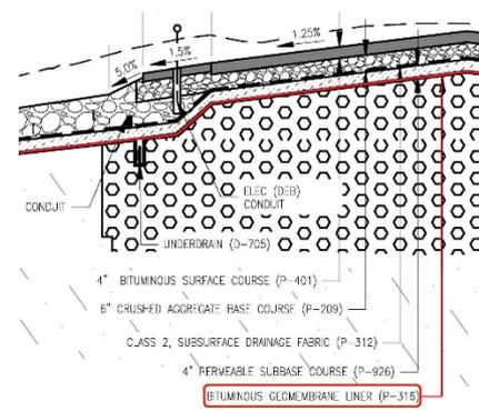
Figure 3. Cross-section under layer of asphalt-concrete
