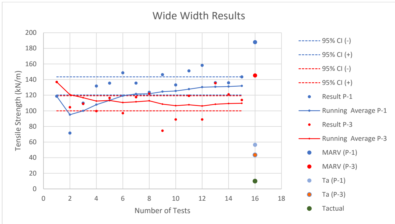
Figure 1: Results of Geogrid Testing of Exhumed Specimens
