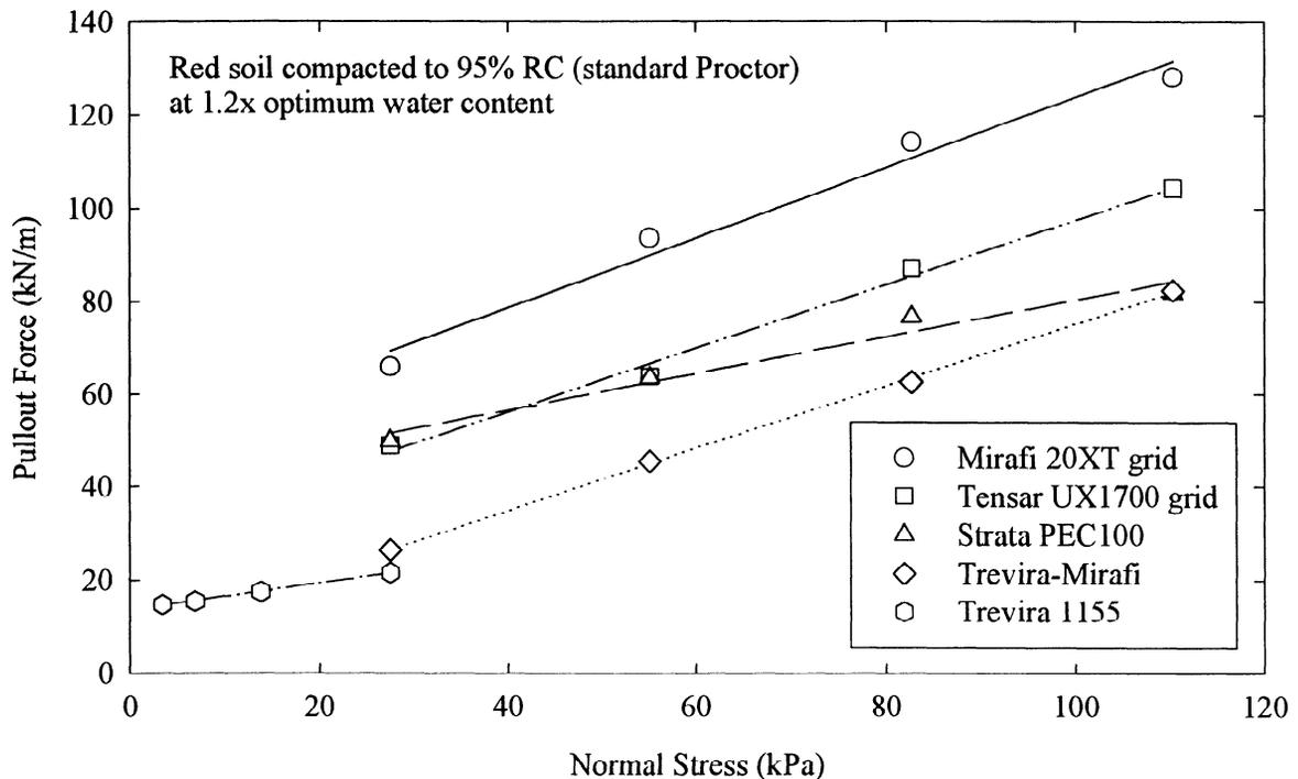
Figure 1. Pullout Test Results
