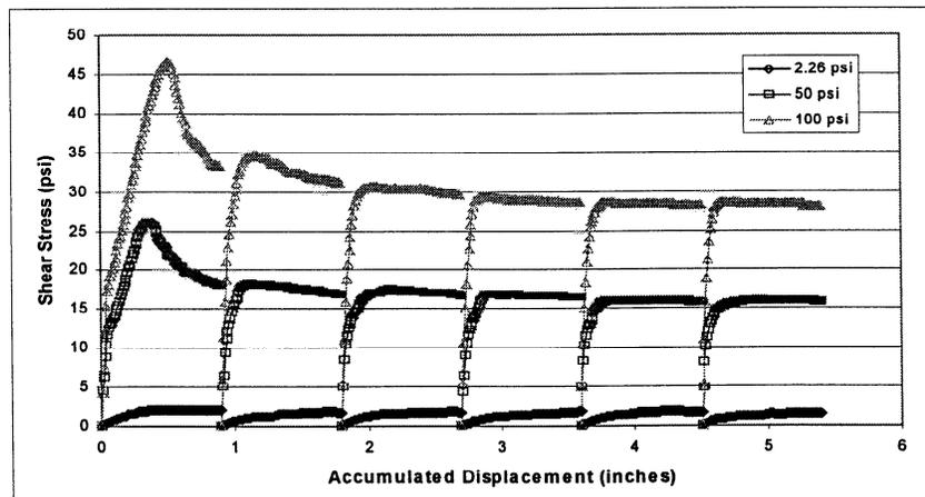
Figure 5. Examples of The Accumulated Displacement Test Results (GMXG/GTNW Interface)
