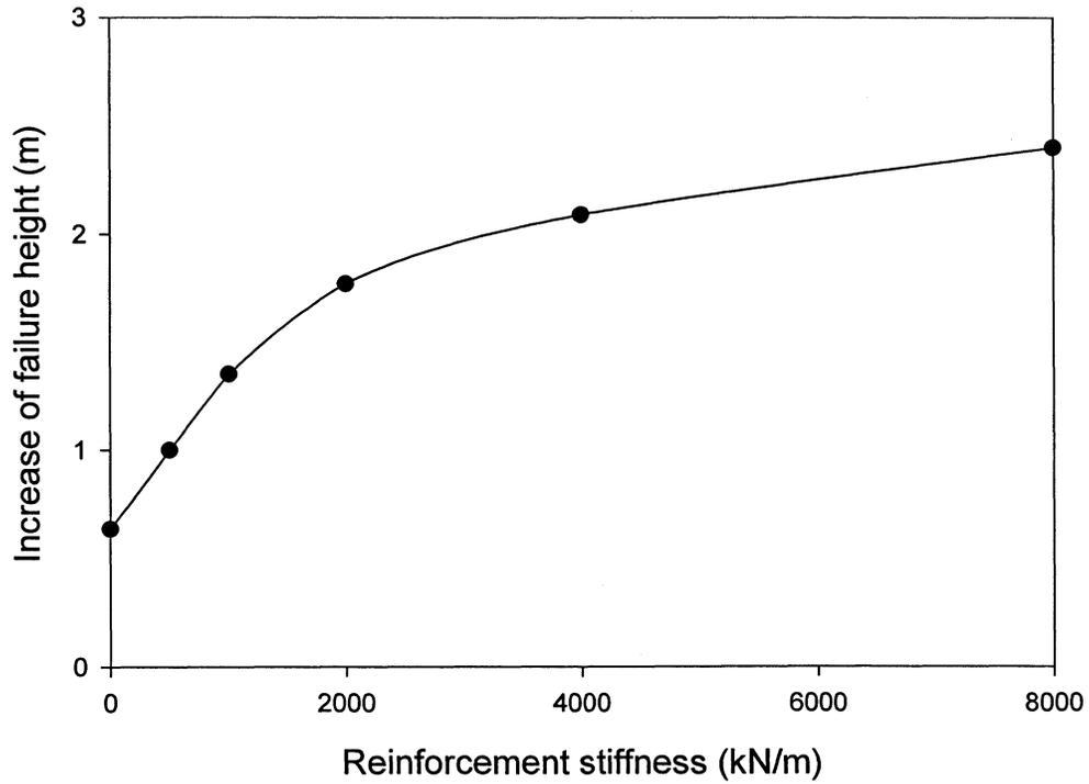
Figure 9. Increase of failure height after 95% consolidation
