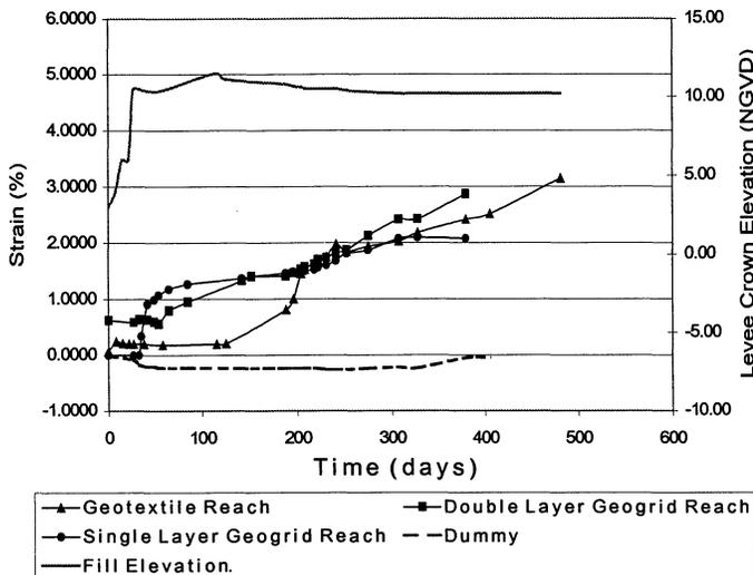
FIGURE 11. Strain vs. Time
