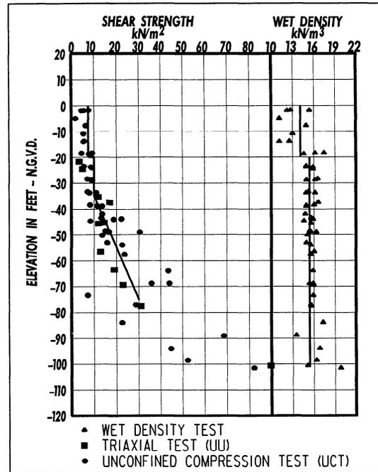
FIGURE 2. Shear Strength Profile
