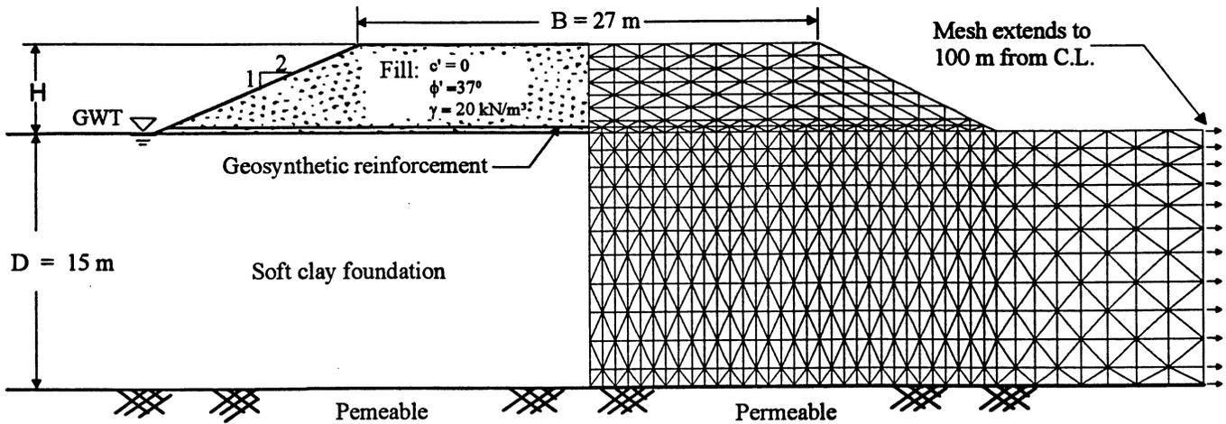
Figure 1. Reinforced Embankment and Foundation
