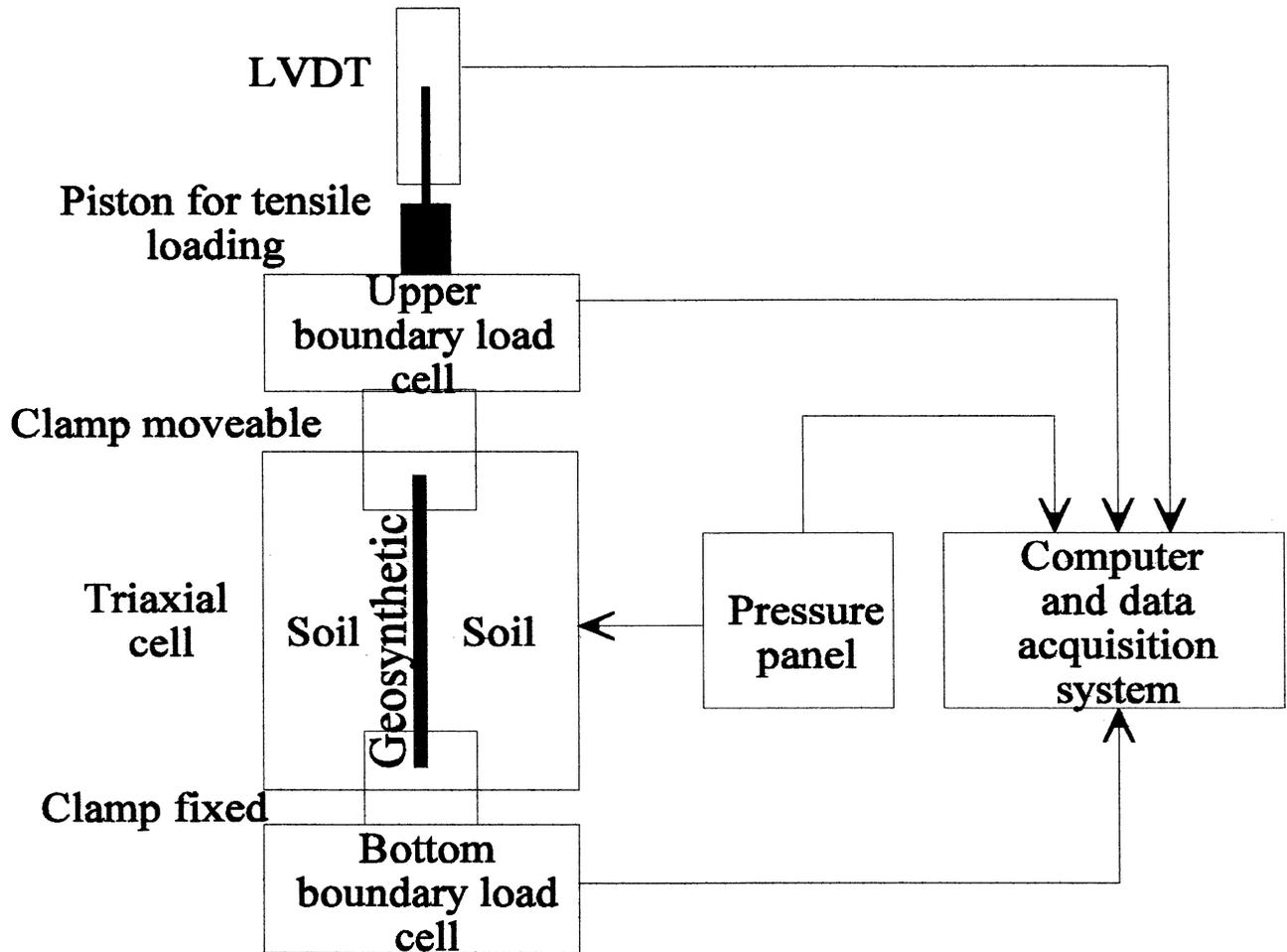
Figure 3 Triaxial system for pullout wide strip testing.
