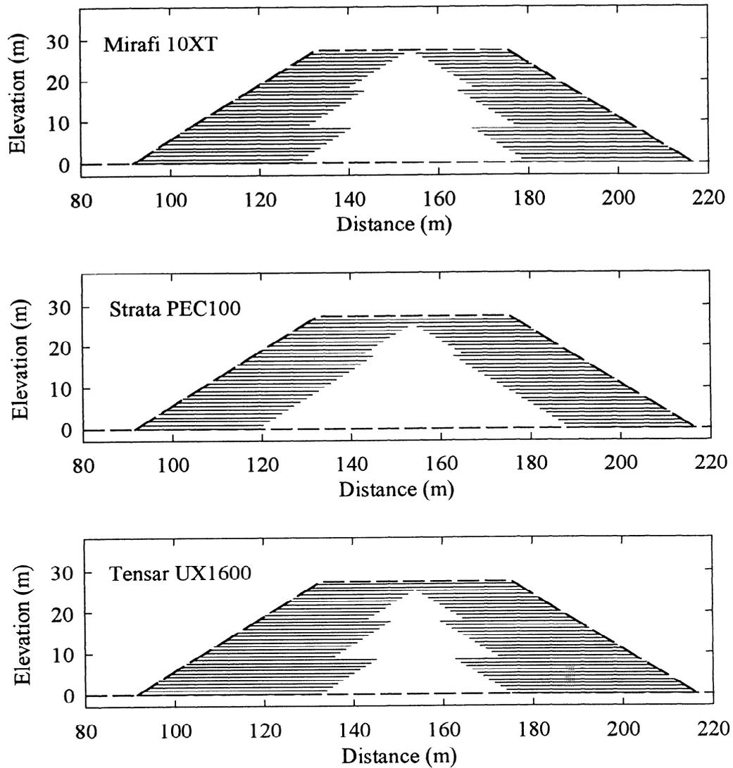
Figure 3. Reinforced Embankment Designs with Uniform Reinforcement Distribution
