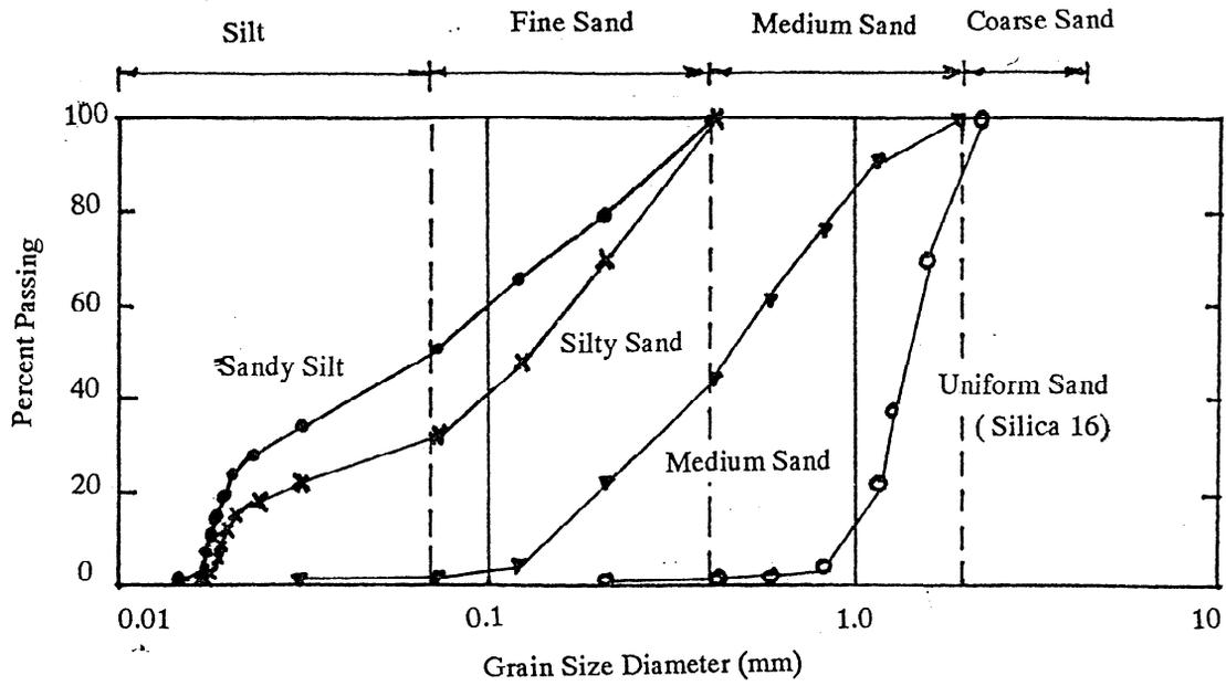
Figure 1. Grain Size Distribution of Test Soils
