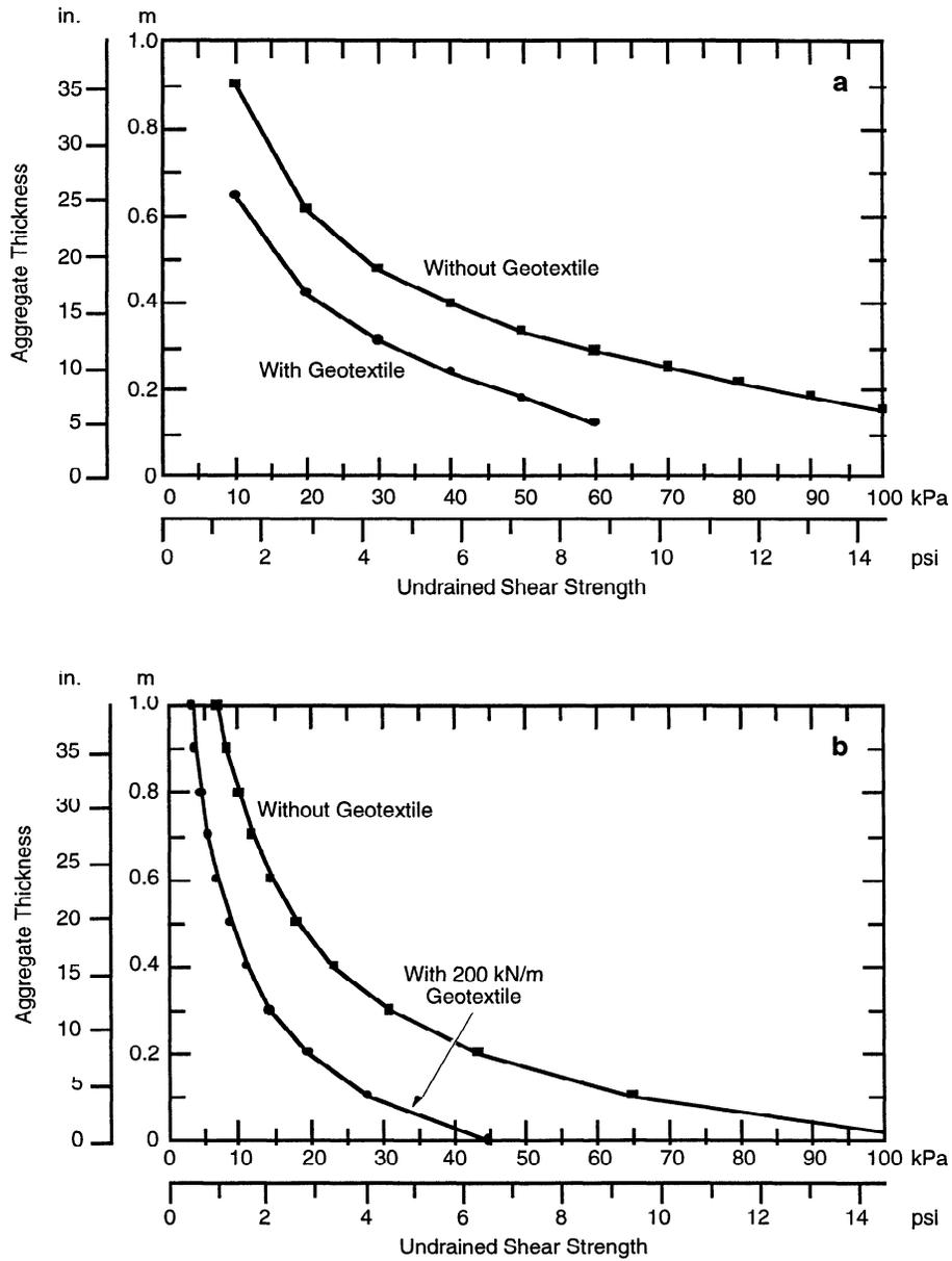
Figure 7: Design curves for static loading for (a) 10-ton dump truck, according to Barenberg (1975) method and (b) Giroud and Noiray (1981) method.
