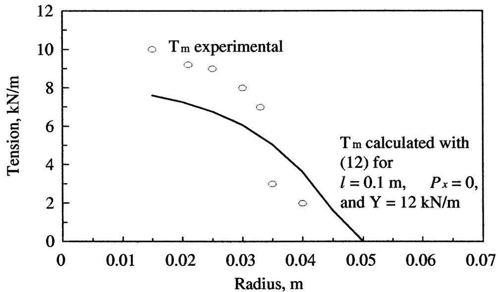
**Figure 5.** Change of tensile stress required for the hole's growth at failure. Unconfined conditions.
