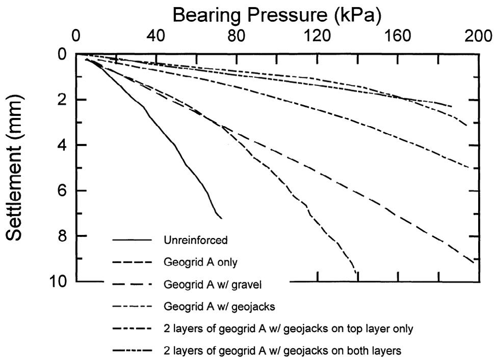
Figure 6 Detail showing initial portion of curves of bearing pressure vs. settlement where Geogrid A was the primary reinforcement
