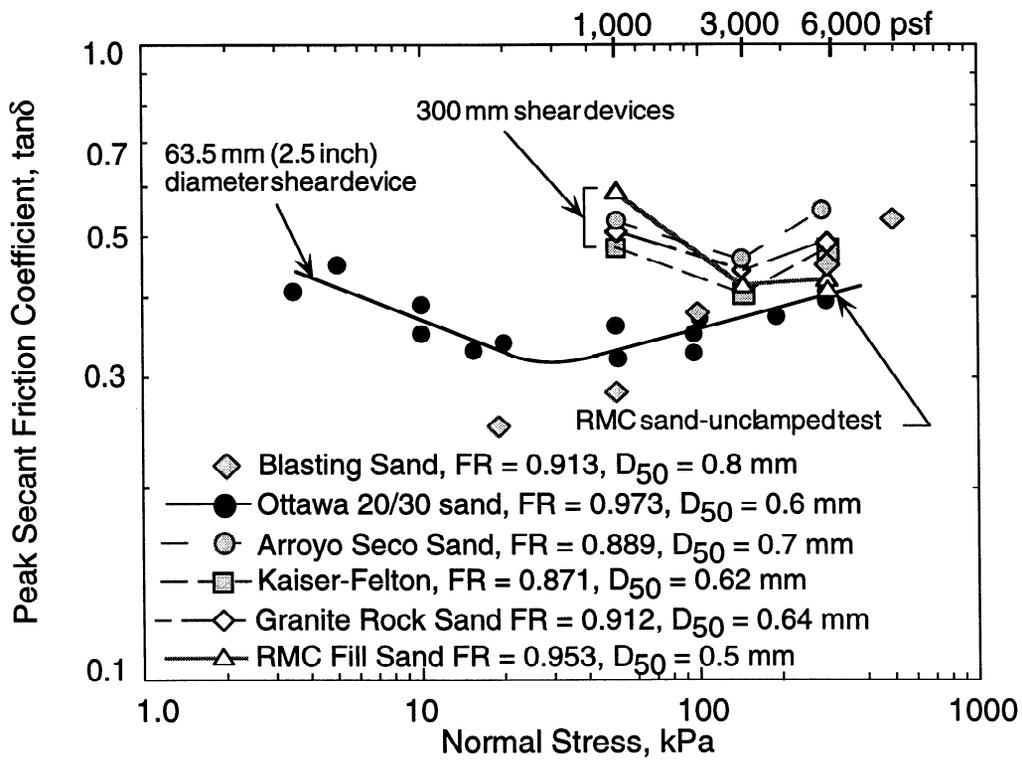
Figure 3. Behavior of Sand/Smooth HDPE Geomembrane Interfaces
