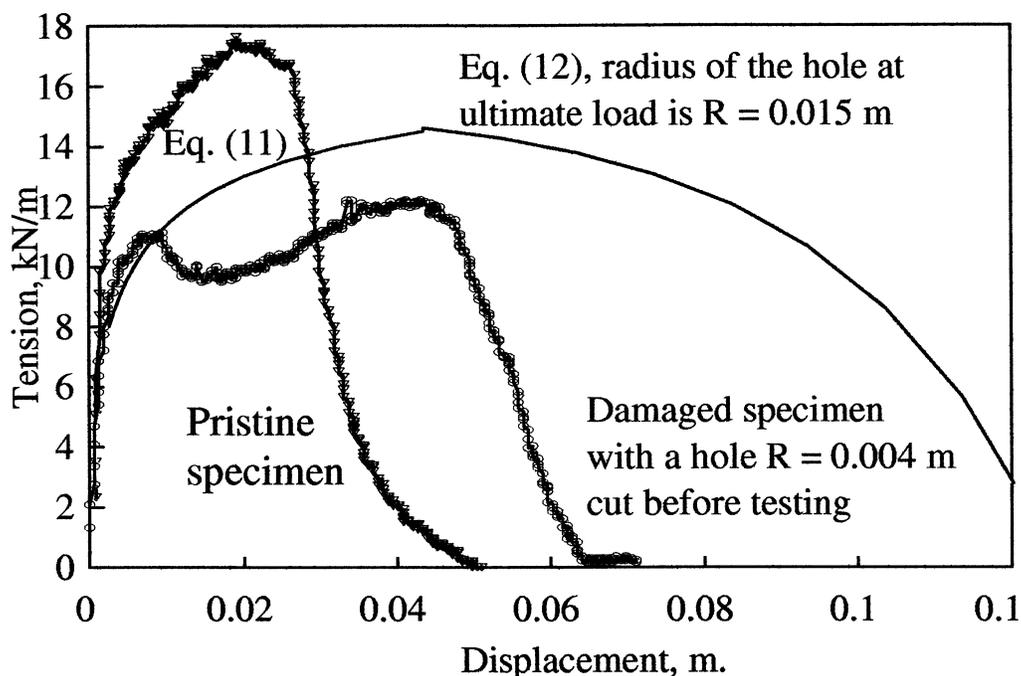
**Figure 8.** Pullout test of pristine and damaged specimens at confining pressure of 140 kPa. Analytical prediction of tensile behavior of a damaged specimen based on unconfined geosynthetic properties,  $R$ , and  $P_x$ .
