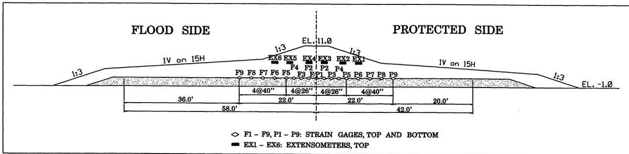
FIGURE 5. Location of Strain Gages and Extensometers
