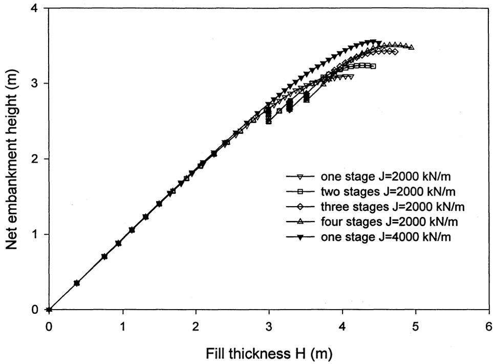
Figure 6. Effect of Multi-stage Construction on Embankment Height
