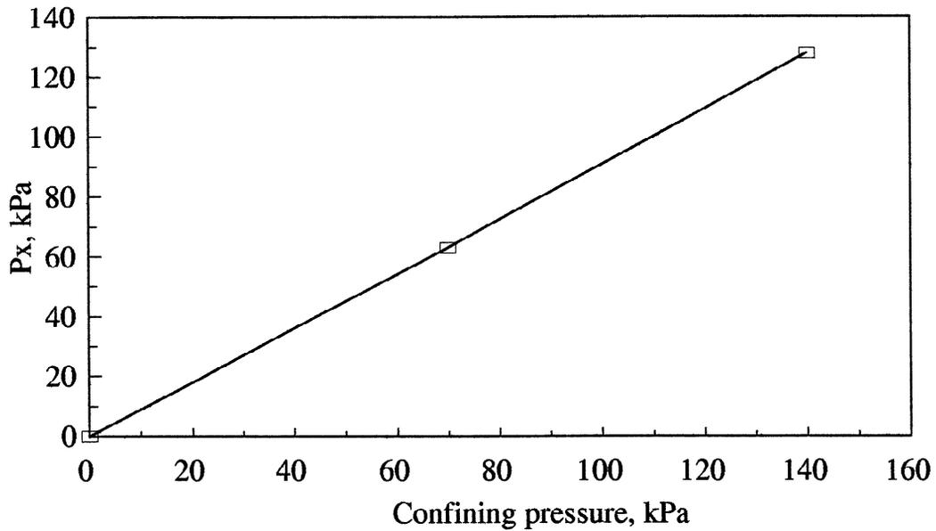
**Figure 7.** Experimental evaluation of the effect of confining pressure on soil-geosynthetic interaction characteristic,  $P_x$ .
