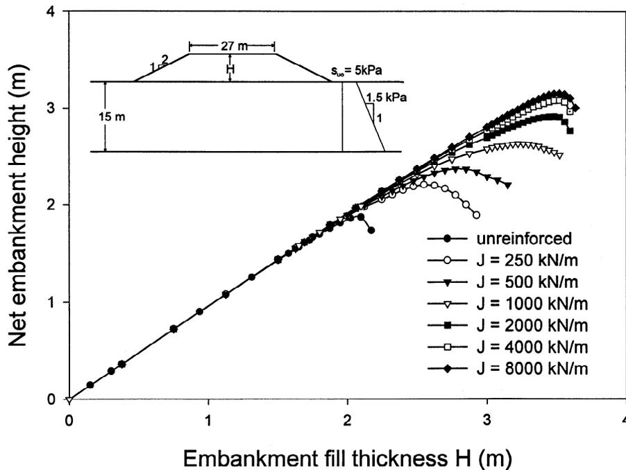
Fig. 2. Variation in Calculated Net Height vs Fill Thickness Under Undrained Conditions
