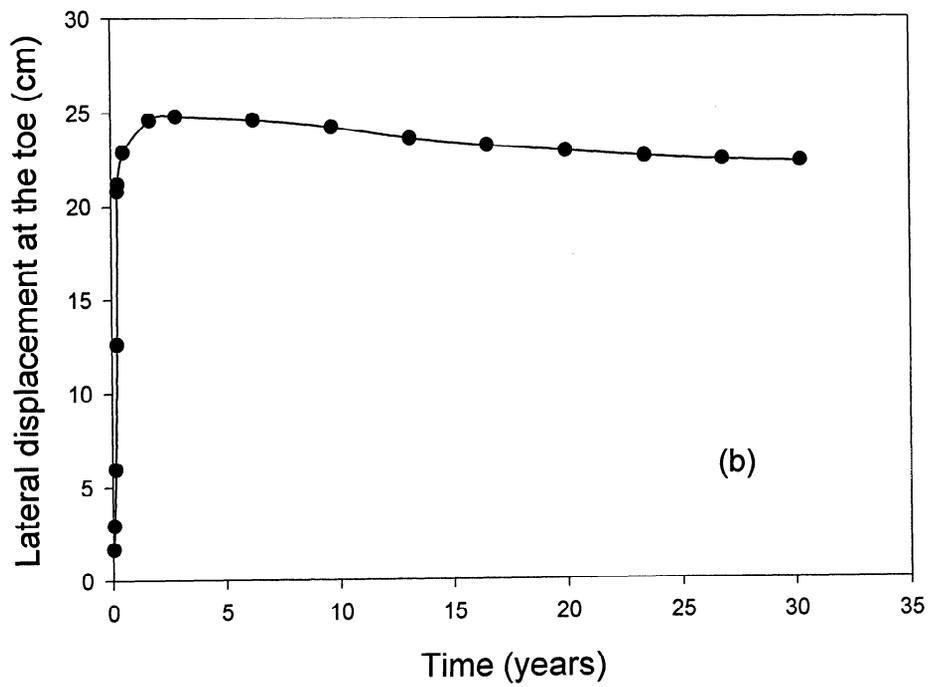
Figure 10. Variation of Maximum Reinforcement Strain and Lateral Displacement at the Embankment Toe with Time: (a) maximum reinforcement strain; (b) lateral displacement
