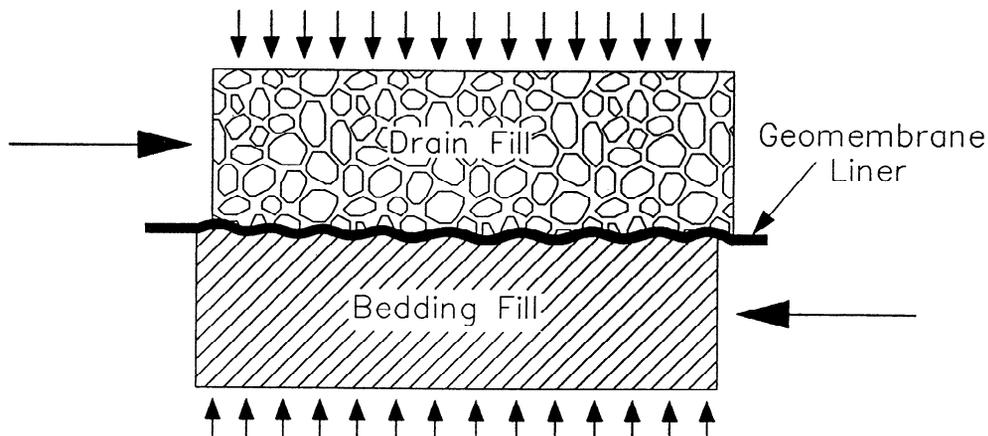
Figure 3. Schematic Diagram of Non-Planar (Dimpled) Direct Shear Test Setup
