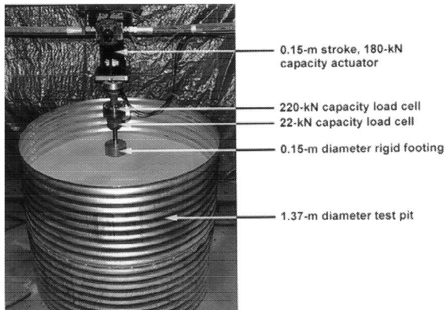
Figure 2 Strain-controlled loading system used in this study
