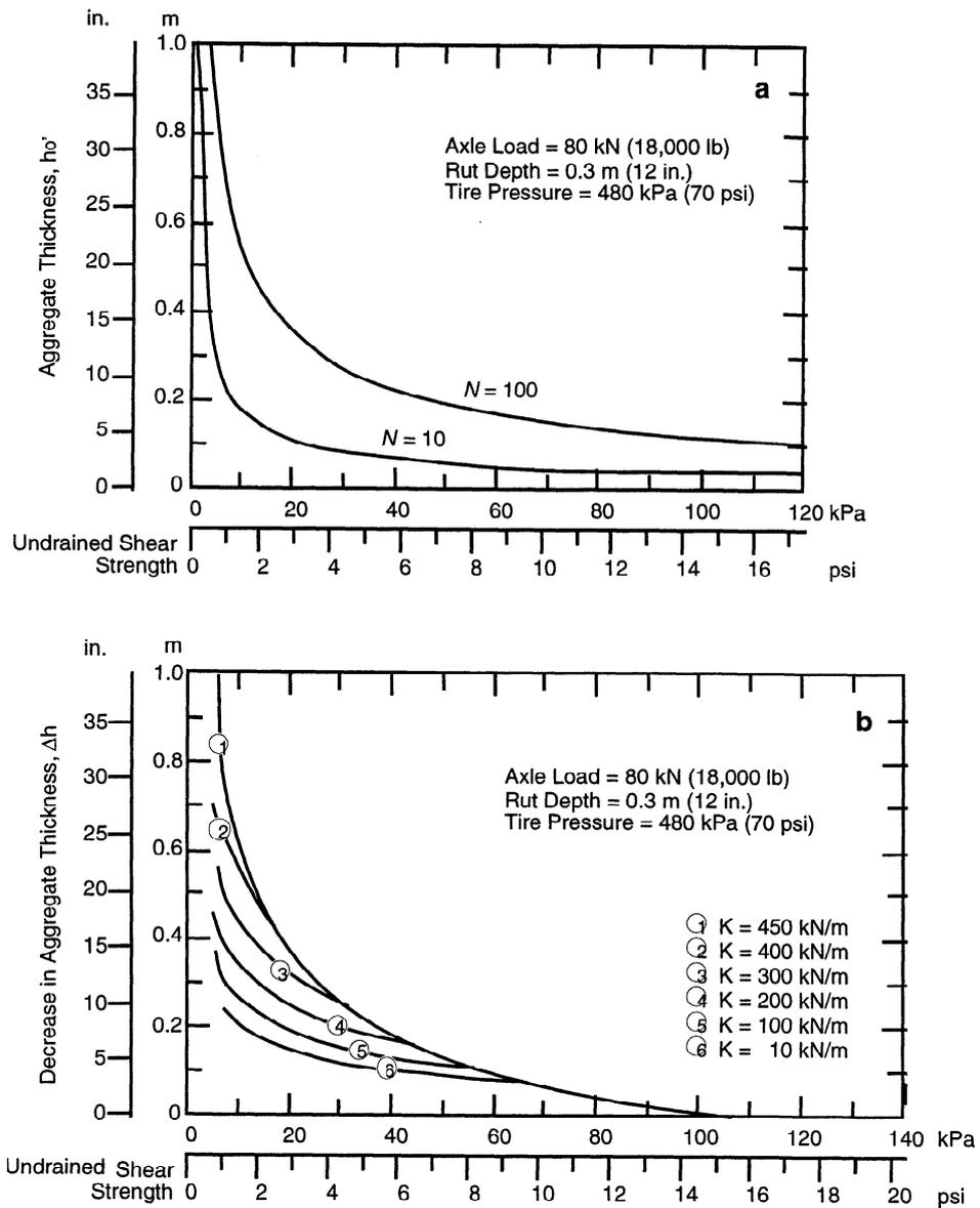
Figure 3: (a) Aggregate thickness,  $h_o'$ , without geotextile ( $N$  is number of applications of axle-load to unsurfaced road); and (b) reduction of aggregate thickness,  $\Delta h$ , resulting from use of geotextile as function of soil cohesion (from Giroud and Noiray, 1981).
