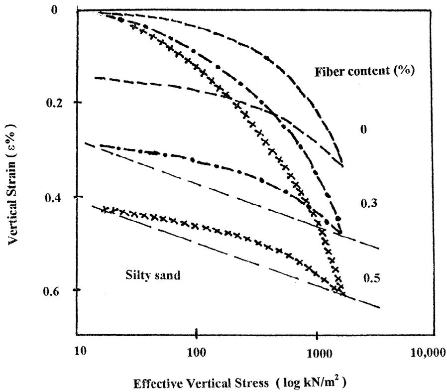
Figure 5. Compression of Silty Sand Specimens in Oedometer
