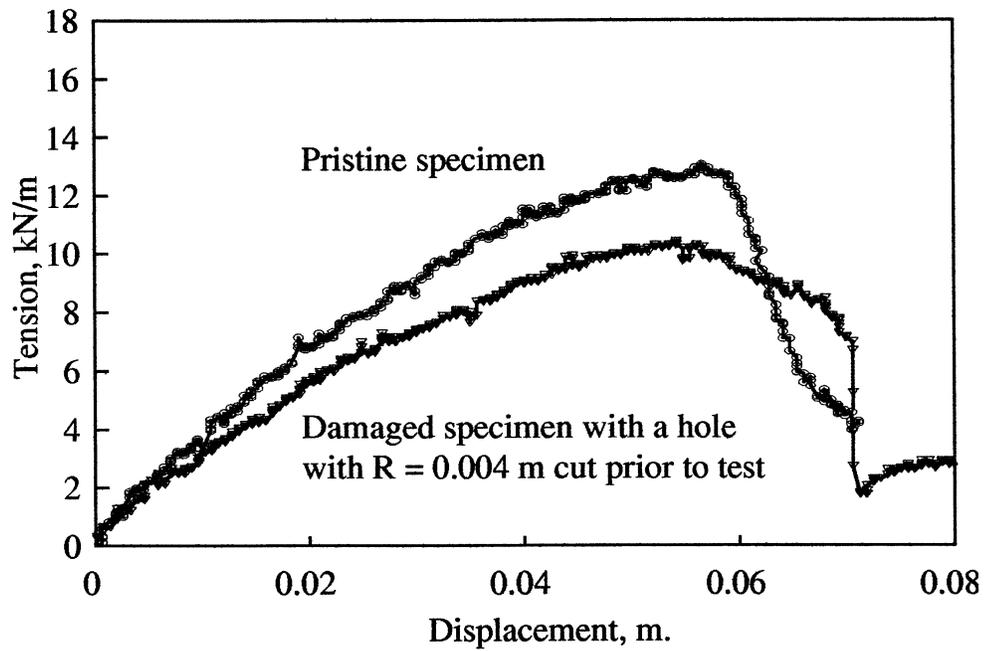
**Figure 4.** Wide strip unconfined test of pristine and damaged specimens.
