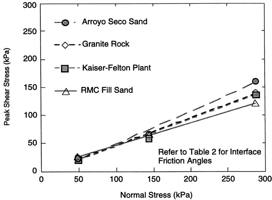
Figure 2. Peak Strength Envelopes from Sand/Smooth Geomembrane Tests
