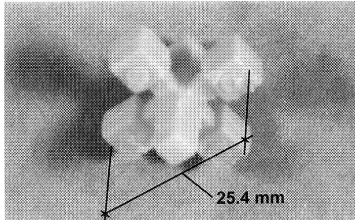
Figure 1 Detail of a single polypropylene-fiberglass geogjack
